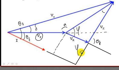
In the figure, a 247.574 volts source delivers 3.96118 kVA at a power factor 0.972502 inductive through a cable with R = 0.07 ohms and X = 6R to a load. Compute: (a) the voltage at the load; (b) the active power of the load; (c) the reactive power of the load and (d) the power factor angle of the load.
