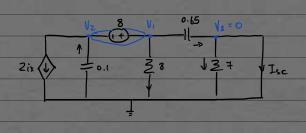
$$\frac{V_1 - V_3}{Zc_2} = \frac{V_3}{7} + I_{SC}$$
